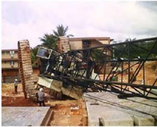
This crane overturned while lifting pre-cast concrete panels. The crane was working on soft ground with a lack of proper cribbing.
