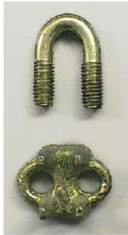
Forged Alloy Steel Notice the expanded saddle
